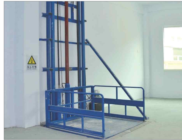
▲ 1 Ton capacity Hydraulic Lift for every unit
